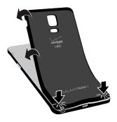
2. Press along the edge of the back cover until you have a secure seal.
